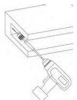
Keyless chuck, female thr. 3/8"-24UNF, capacity 1,5-10mm, Porta's model number LD10F38R **Model PML**
